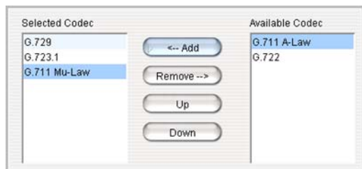
Figure 206. Codec negotiation example: SIP devices on a WAN
