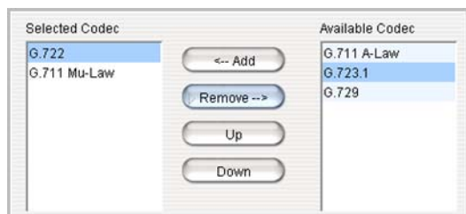
Figure 205. Codec negotiation example: SIP devices on a LAN
